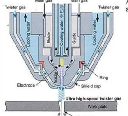
A powerful downward spiral flow around the plasma arc reduces dross. (US Patents No.6268583, No.6222154)
