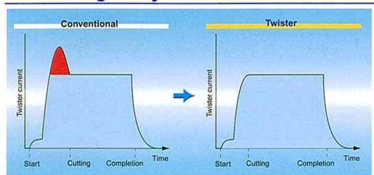
Due to the quick arc change, current overshoot on ignition has been curbed. Thus, the life of consumable parts has been greatly extended. (US Patent No.6933463)
