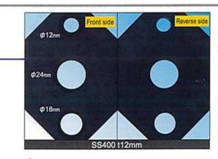
The arc mode has been optimised matched to configurations by using main gas flow control. This has greatly improved cutting quality. (US Patent No.6248972)
