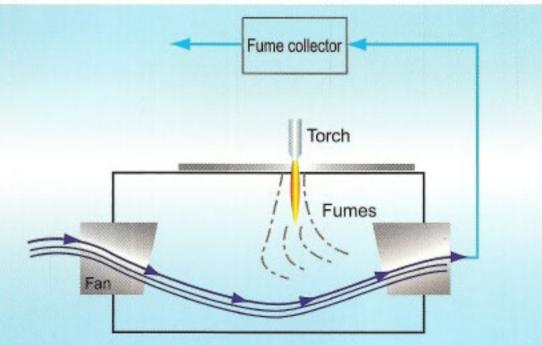
Effective fume (dust) collection is achieved by the push-pull system and zoned fume collection system limited to the work area. This greatly improves working environment. (US Patent No.6664495)
